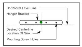
**STEP 2:** Mark a horizontal level line on the wall at the height determined in step 1. Now make a mark along this horizontal line at the desired centerline location of the sink.
