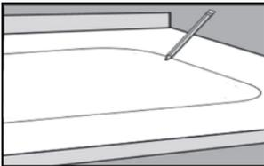
**STEP 2:** Using tape lines or crayon, transfer the dimensions you noted in **Step 1** onto the countertop surface, positioning and aligning them in the desired location of the installed sink. These markings should now represent the sinks outer perimeter edges. **Cautionary Note: Make sure to radius all corner markings as necessary and verify your dimensions and markings!**
