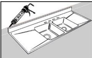
**STEP 7:** Place the sink back into the countertop opening and position it in its final location. Apply a continuous bead of the appropriate colored (we recommend the sinks finish color be used) kitchen & bath adhesive sealant around the entire perimeter of sinks flange where it meets the countertop surface. Remove and cleanup excess sealant and allow curing time per the sealant manufacturer's recommendation.
